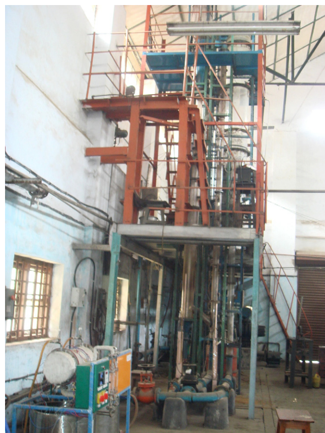
Fig. 3. Photographic view of the experimental set-up of the riser of a circulating fluidized bed.
